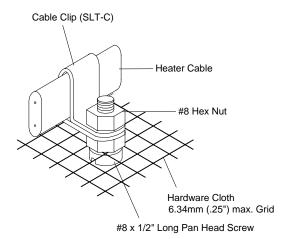
**Flat Roof** - Adhesive (not furnished) should be used to bond clips studs to the flat surface. The roof surface should be clean at the bonding locations. **Do not penetrate flat roofs with screws or nails as leaks may develop.** Allow the adhesive to cure to full bonding strength before attempting to install the cable and clips.
