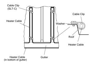
**Metal Roof** - Fasten with sheet metal screw using neoprene sealing washer. If washers are not available, coat screw and upslope edge of clip with silicone sealant. Exact cable spacing may vary depending on the rib design of the roof. Typically trace every other rib.
