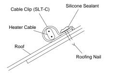
Asphalt/Shake Shingle Roof - Fasten with nail, coat nail head and upslope edge of clip with silicone sealant.
